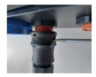
Removal is not possible without tools. You will need a release tool, e.g. a screwdriver. Use the screwdriver to press into the opening on the side of the plug. The plug can now be released by pulling gently on the plug housing. Once the plug has been pulled out correctly, the black locking pin remains in the socket housing of the ONgineer charging station and ensures that it locks again when the plug is reinserted.
